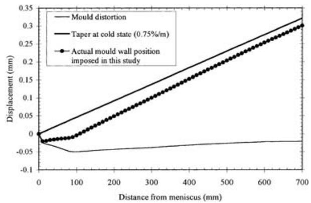
**6 Profiles of mould distortion and taper used in present model**
