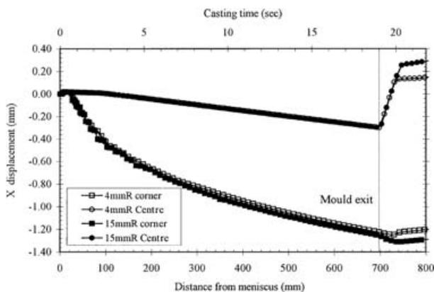
16 Evolution of billet surface displacement showing bulging below mould exit with given corner radii *R*
