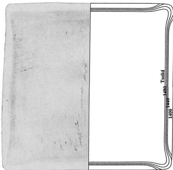
12 Comparison of calculated and measured solid shell thicknesses: C = 0.04 wt.%, 285 mm below meniscus, casting speed 2.2 m min<sup>-1</sup>
