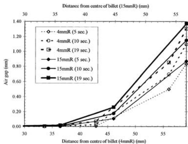
20 Evolution of air gap size profiles with given corner radii
