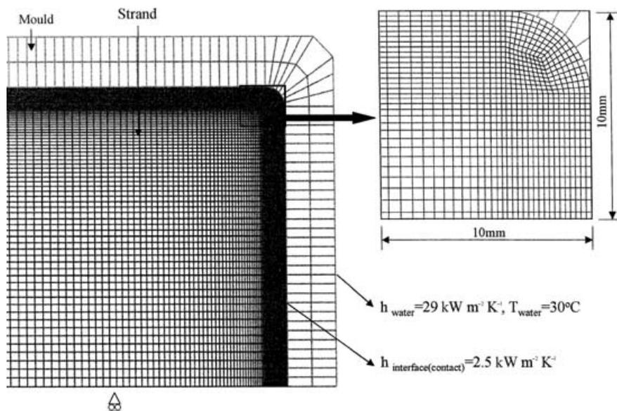
7 Finite element mesh of two-dimensional horizontal quarter domain for billet strand and mould and its boundary conditions:  $h$  heat transfer coefficient,  $T$  temperature
