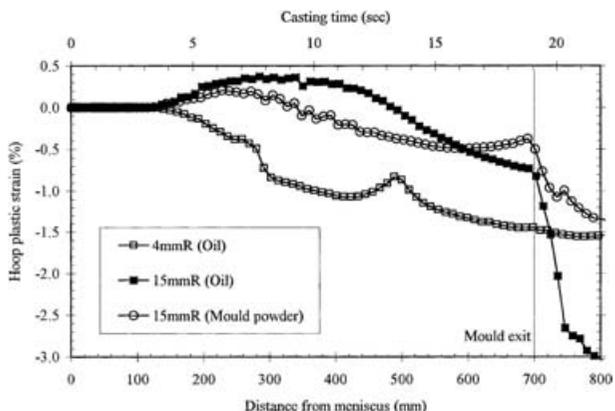
22 Evolution of hoop plastic strain at 1 mm below billet corner surface for given casting conditions
