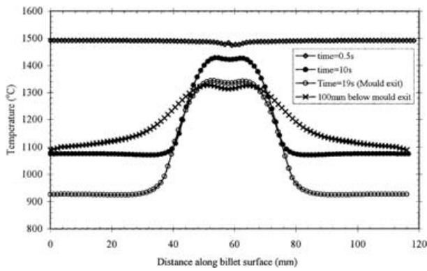
15 Surface temperature profiles along 4 mm corner radius billet at given times
