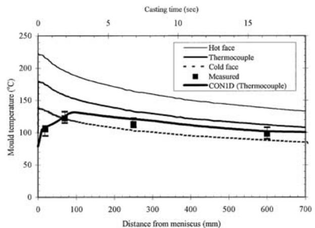
10 Comparison of measured and calculated mould temperatures
