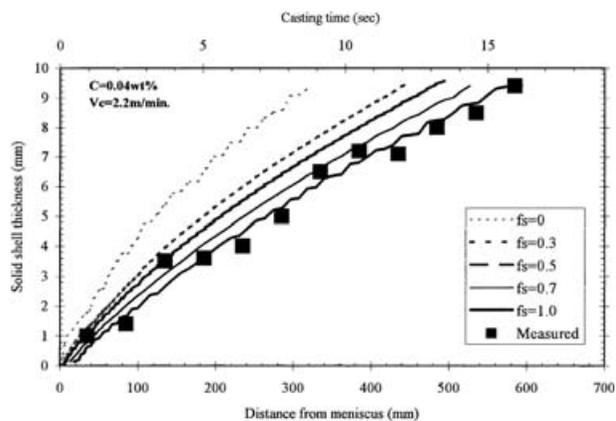
13 Comparison of measured and calculated solid shell thicknesses with casting time: V<sub>c</sub> casting speed
