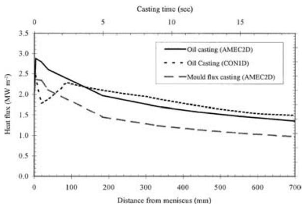
11 Heat flux profiles down mould for given casting conditions and models
