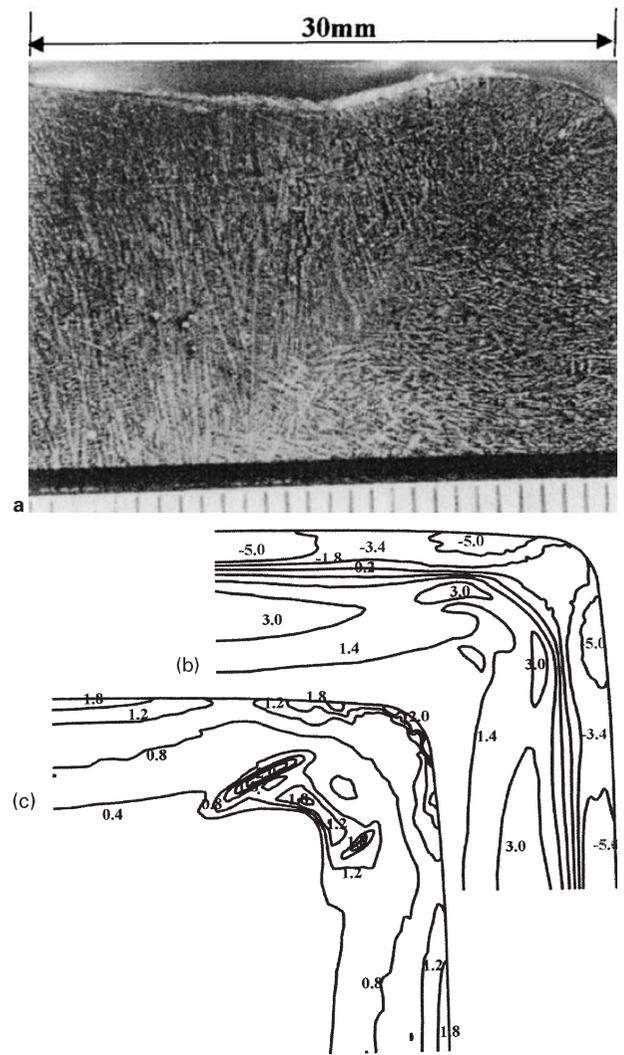
a microstructure of off corner crack; b hoop stress distribution; c equivalent plastic strain contours
